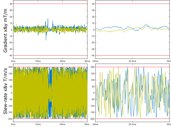
Figure 4: Gradient (top) and slew-rate (bottom) plots of the learned k -space trajectory with radial initialization for N_{\text{shots}} = 16 . The right column depicts a zoom-in portion. The red lines are the constraints used in the optimization: maximum gradient G_{\text{max}} = 40 \text{ mT/m} , maximum slew-rate S_{\text{max}} = 200 \text{ T/m/s} .
